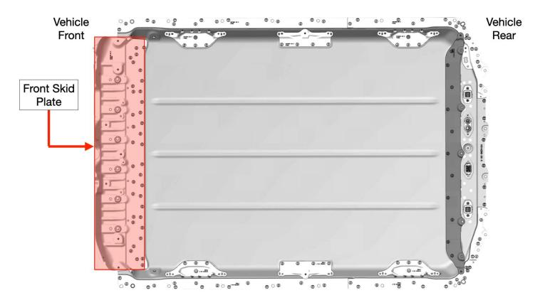
Figure 9 - Front skid plate location
