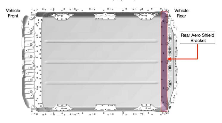
Figure 19 - Rear aero shield bracket
