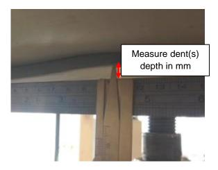
Figure 8 – Measuring the depth of enclosure damage
