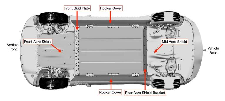
Figure 4 - Structural HV battery assembly key components
