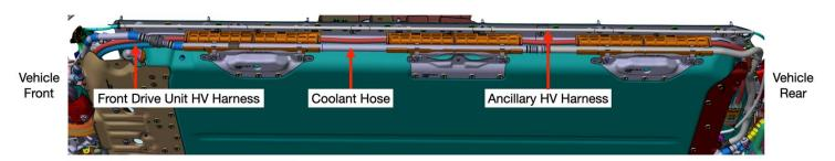
Figure 13 - Left side of HV battery
