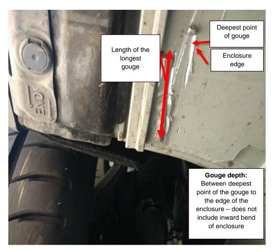
Figure 17 – Gouges in the baseplate
