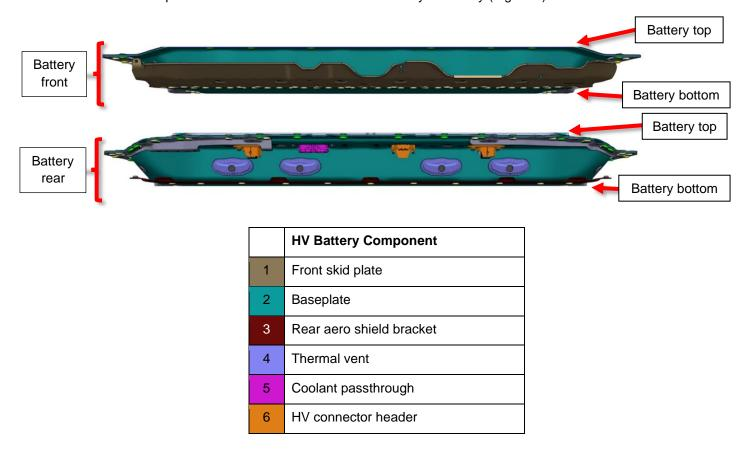
Figure 7 – Structural HV battery front and rear
