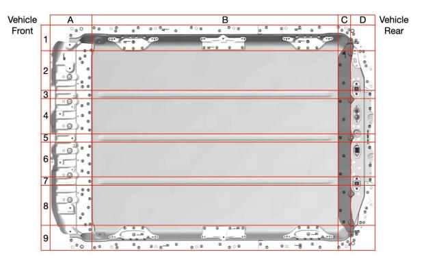
Figure 5 – Structural HV battery underside grid layout
