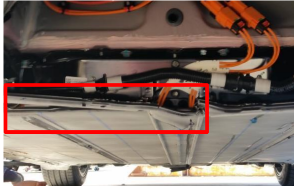
Figure 9 – Torn front skid plate
