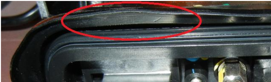
Figure 4 (Seal deformed outwards)
