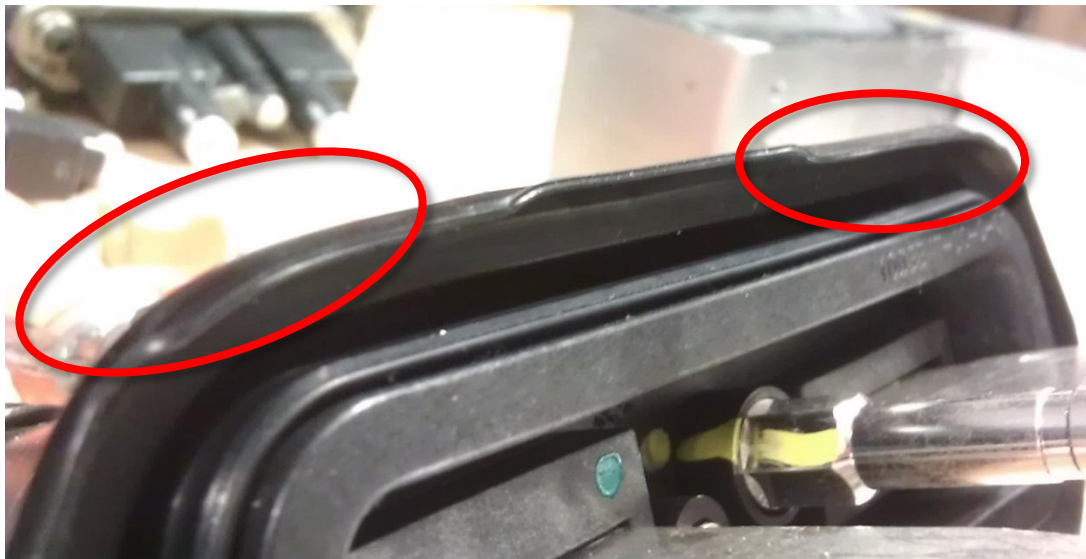
Figure 5 (Seal deformed inwards)
