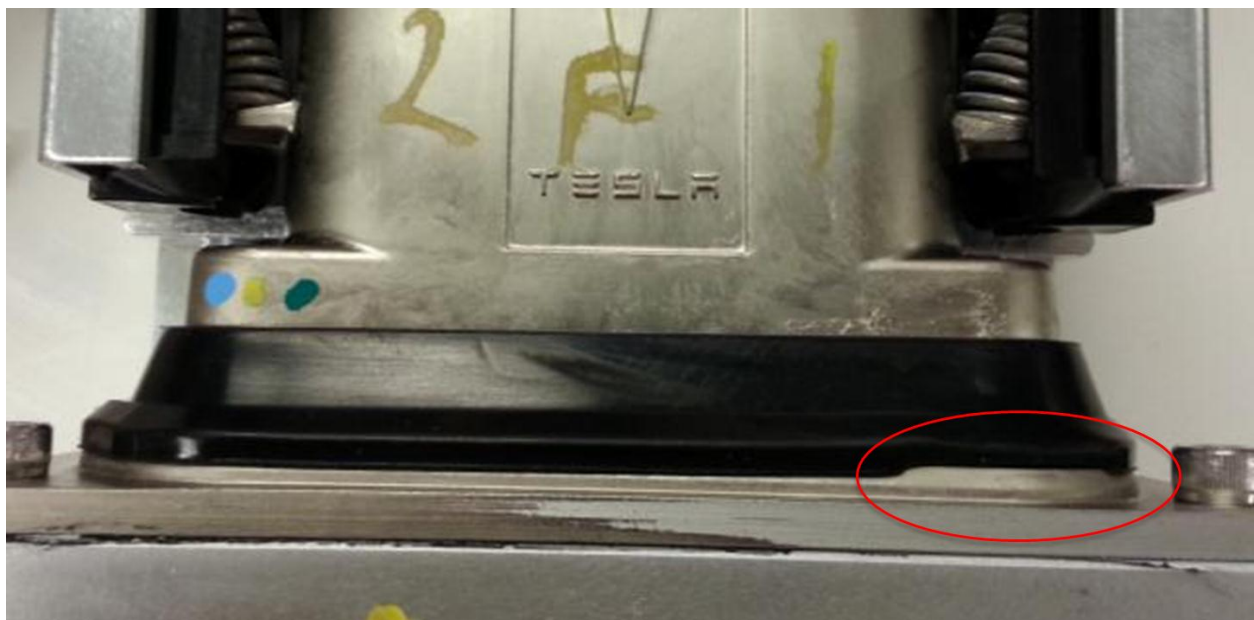
✗ Incorrect – Skirt seal caught on base Figure 18
