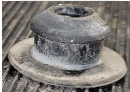
Figure 4 – Pass: Limit of allowable salt deposits
