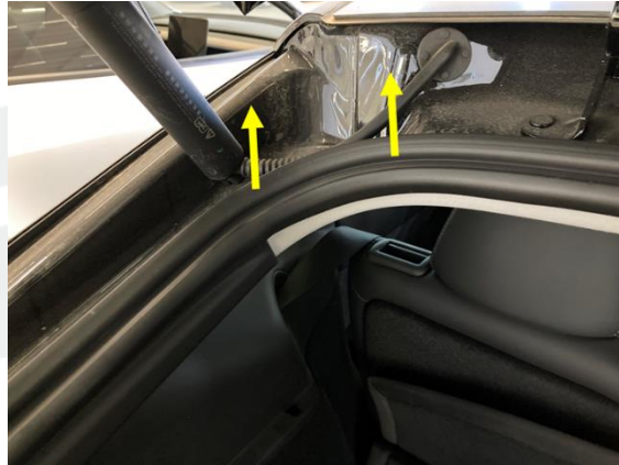
Figure 1 – Strut might not be connected to the body as shown
