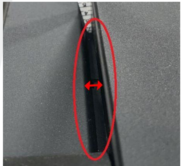
Figure 3 – Gap Between Water Management Slat and Tonneau Applique (Red Arrow); Water Management Channel Exposed
