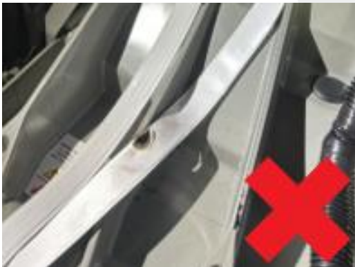
Figure 5 – Example damage at the front passenger section of the FFC
