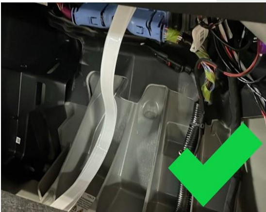
Figure 17 – Correctly routed through LH channel
