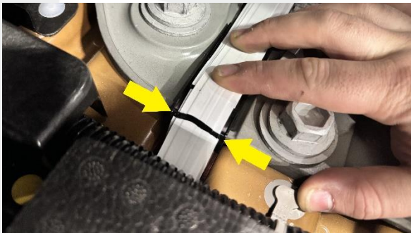
Figure 22 – Mark FFC at rear edge of harness guide
