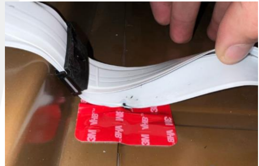
Figure 6 – Example damage at the rear passenger section of the FFC
