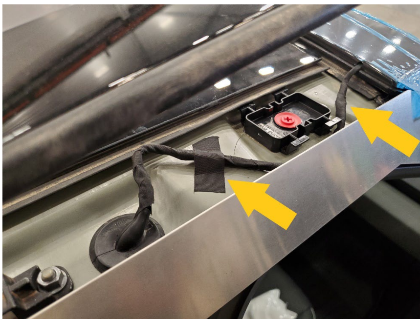
Figure 31 – Correct harness routing
