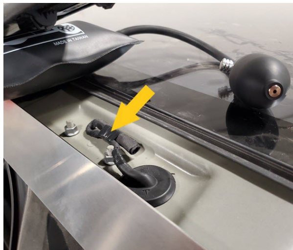
Figure 1 – Roof accessory jumper harness
