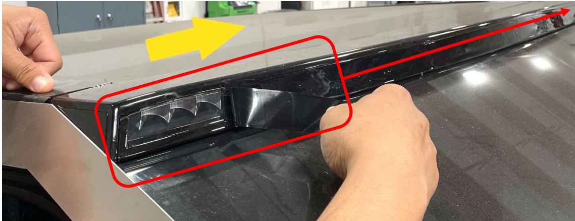
Figure 32 – Blackout film tape removal
