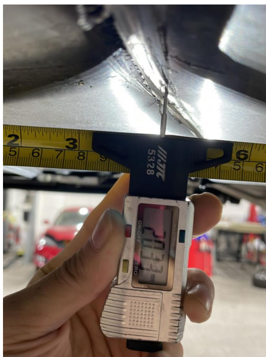
Figure 13 – Dent exceeding the maximum threshold
