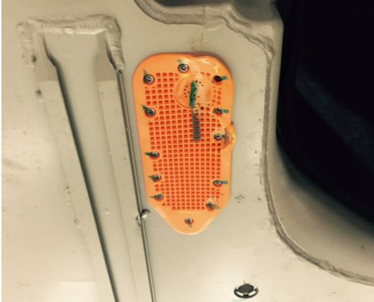
Figure 9 – Light plastic deformation of the front baffle cover
