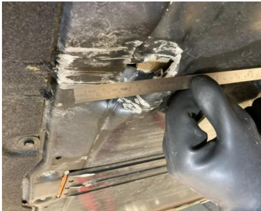
Figure 8 – Enclosure rupture exposing internal components
