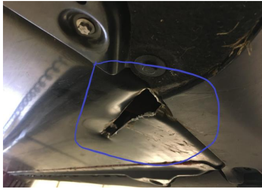
Figure 6 – Enclosure rupture exposing internal components
