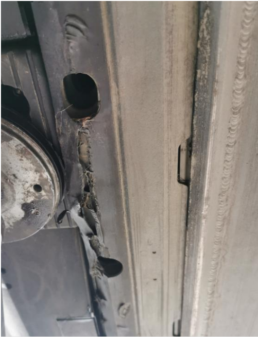
Figure 10 – Side ski plastic cover damage
