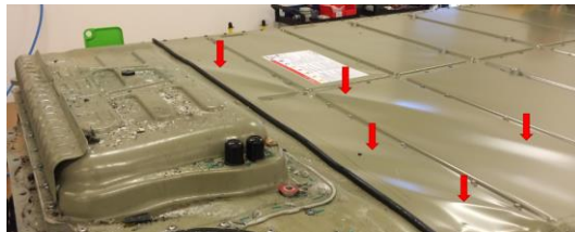
Figure 16 – Enclosure top cover visually warped
