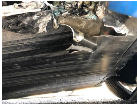
Figure 2 – Enclosure underside tear exposing internal cells
