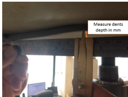
Figure 11 – Dent exceeding the maximum threshold
