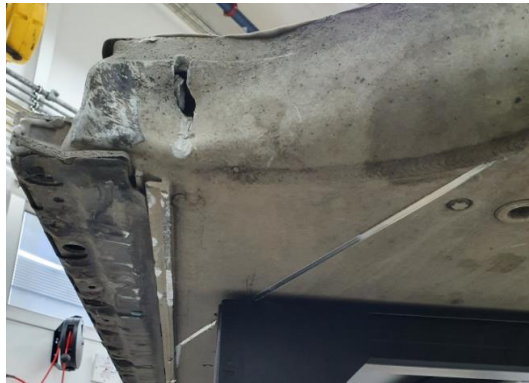
Figure 7 – Enclosure rupture exposing internal components
