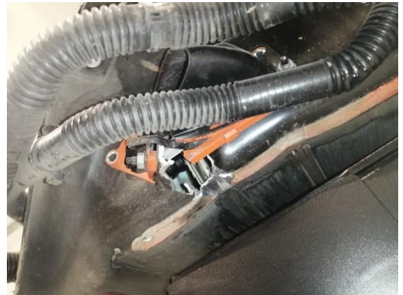
Figure 8 – Enclosure rupture exposing internal components
