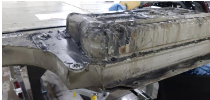
Figure 20 – Soot-like discoloration on enclosure
