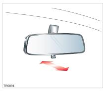
Push the lever on the underside of the mirror to dip the mirror. Pull the lever to restore normal visibility.
