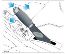
To release the hand brake, pull the lever up slightly, depress the button (shown in illustration) and fully lower the lever. The warning indicator will extinguish and the Touch Screen will display a Drive screen.
