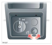
The control for the instrument panel lighting is located on the left-hand side of the dashboard. When instrument panel lighting is turned on using the adjacent switch, you can adjust the amount of backlighting on the instrument panel, the Touch Screen, and the center console by turning this knob clockwise to increase the backlighting and counter-clockwise to decrease the backlighting.
