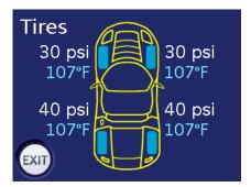
A blue wheel indicates an acceptable operating pressure for the tire.
