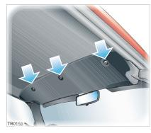
13. Starting with the bolt in the center, tighten the three bolts to secure the trim panel. Do not overtighten.
