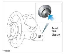
The TRIP display shows the miles traveled since the trip display was last reset. To reset the trip display to zero, press and hold the button on the side of the steering column for about one second.
