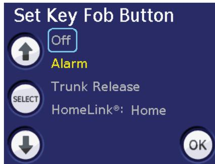
You can program the third button on your key fob to activate the vehicle's alarm, open the trunk, or operate a HomeLink® device.
