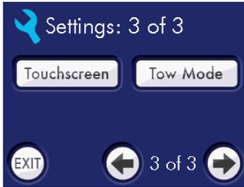
4. Touch **Tow Mode**, then touch **OK** to confirm. The Touch Screen displays the following message indicating that the vehicle is in Tow Mode.
