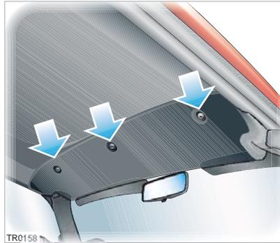
13. Starting with the bolt in the center, tighten the three bolts to secure the trim panel. Do not overtighten.
