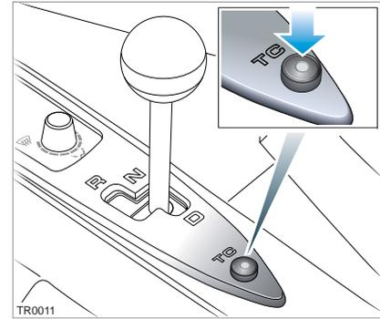
Under normal conditions, traction control should be left on. The system should only be switched off in circumstances where you deliberately want the wheels to slip. As soon as the circumstances requiring you to switch traction control off have passed, press the switch to turn traction control back on.
