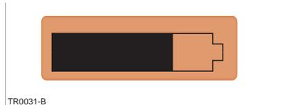
The size of the filled region within the battery icon provides a visual indicator of the amount of charge remaining in the Battery.
