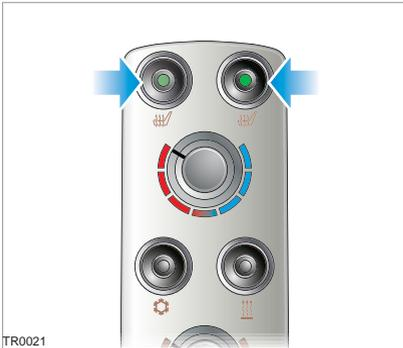
Press the respective button to operate the required seat heater. The seat heaters can be operated at two different levels:
