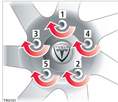
4. Using a torque wrench, fully tighten the bolts in the sequence shown to 77 lbft (105 Nm).
