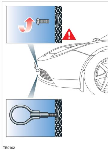
1. Retrieve the recovery eye from the tool kit located in the trunk. See Tool kit components, page 10-2.
