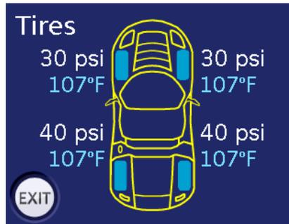
A blue wheel indicates an acceptable operating pressure for the tire.
