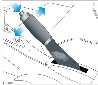
To release the hand brake, pull the lever up slightly, depress the button (shown in illustration) and fully lower the lever. The warning indicator will extinguish and the Touch Screen will display a Drive screen.
