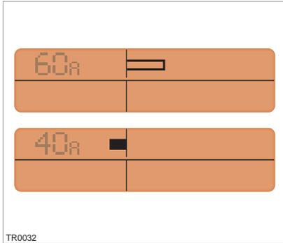
The extending bar on the top right of the LCD is a visual indicator of the amount of and direction of the current:
