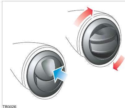
Press the thumb depression to open the vents and rotate to direct the air. The vents on each side of the dashboard can be adjusted to direct air onto the side windows.
