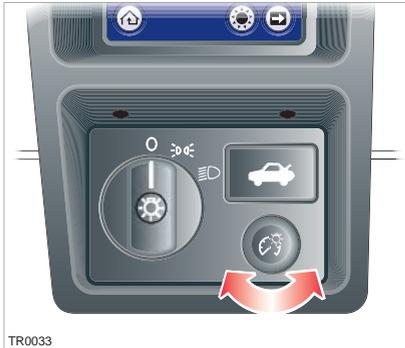
The control for the instrument panel lighting is located on the dashboard below the Touch Screen. When instrument panel lighting is turned on using the adjacent switch, you can adjust the amount of backlighting on the instrument panel, the Touch Screen, and the center console by turning this knob clockwise to increase the backlighting and counter-clockwise to decrease the backlighting.
