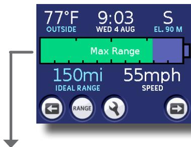
Touch this Battery image to change the vehicle's mode directly from this screen.
