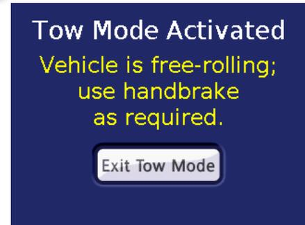
To prepare for safe transportation, Tow Mode disengages the transmission lock needed to move the vehicle when it is turned off. Damage can occur if you move the vehicle (when turned off) without activating Tow Mode. This damage is not covered by the New Vehicle Limited Warranty. For details, see the Roadside Assistance Guide, provided in your owners package.
