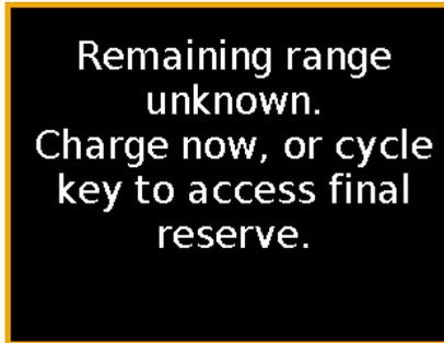
To access final reserve, turn the key to the ACC position then back to the ON position. When you use this feature, the Touch Screen no longer displays warning messages and no longer provides an estimated range.
