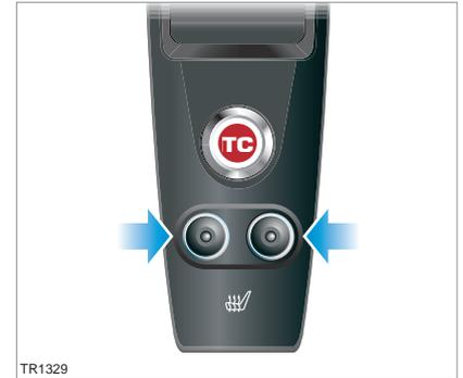
remains illuminated until either the seat heater is manually turned off or the key is turned to the OFF position.
