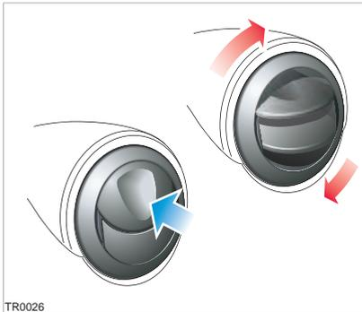
**Note:** When you open the face level vents, airflow to the foot and windshield vents is reduced.
