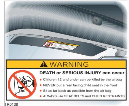
Airbag warning information is printed on the driver's and passenger's sun visor.
