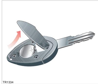
notice a deterioration in performance. For example, you'll gradually need to be closer to the vehicle to operate the key fob.
