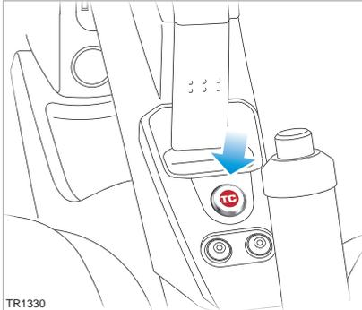
Under normal conditions, traction control should be left on. The system should only be switched off in circumstances where you deliberately want the wheels to slip. As soon as the circumstances requiring you to switch traction control off have passed, press the switch to turn traction control back on.
