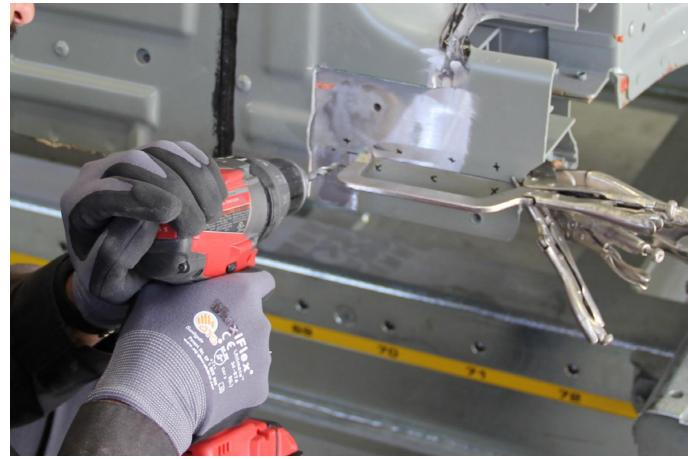
Use a drill with the adjusted countersink cage assembly to countersink the holes in the repair area.
