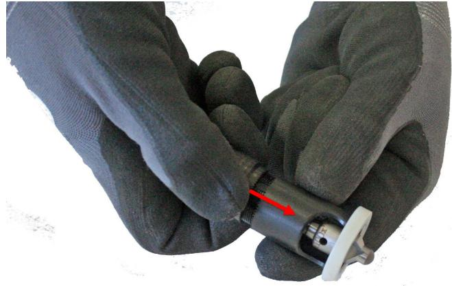
5. Check the depth setting by pushing the shaft forward to the limit of its extension. Repeat steps 2 on page 11 through 4 on page 13 until the cage is in the desired position.
