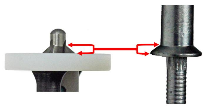
5. Install the countersink cage assembly onto the drill.
