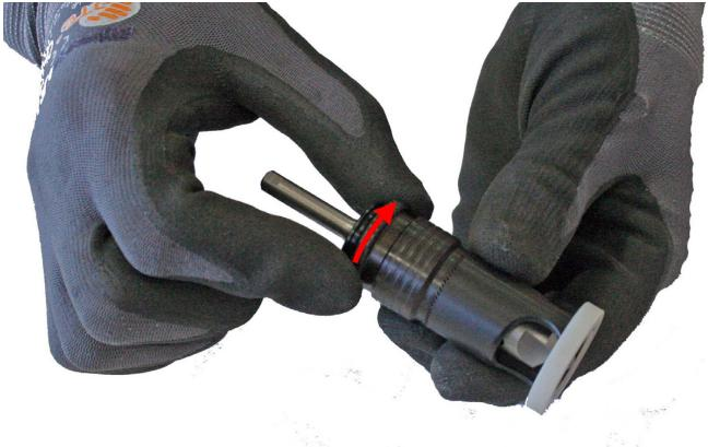
2. Pull the chuck back to disengage it from the cage.
