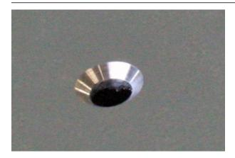
A correctly countersunk hole allows the top of the installed rivet to sit flush to the surface of the surrounding material.
