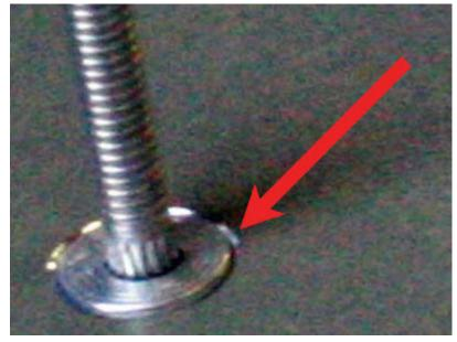
• If the rivet head protrudes above the surface of the material, adjust the countersink cage setting, as described in Adjusting the Depth of the Countersink Hole on page 10 and then repeat Step 7 on page 8 until the rivet head is flush with the surface of the material.
