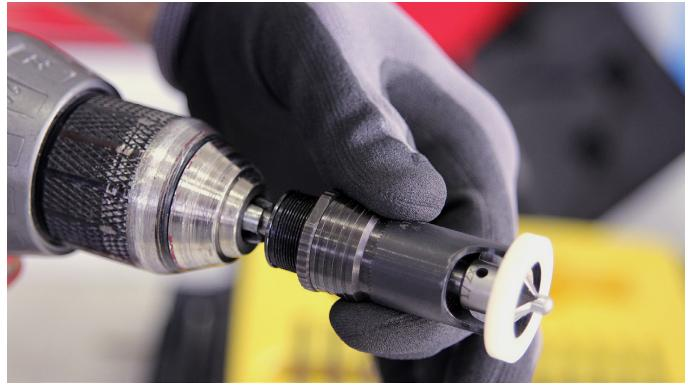
6. Use the drill with the countersink cage assembly to countersink the pilot hole drilled previously (Step 1 on page 4).
