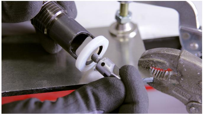
4. Compare the adjustment of the countersink cage assembly to the head of the countersunk rivet to be installed. **NOTE:** The distance that the angled portion of the countersink bit protrudes from the nylon foot when the shaft is fully extended should be slightly less than the distance of the angled portion of the countersunk rivet head.
